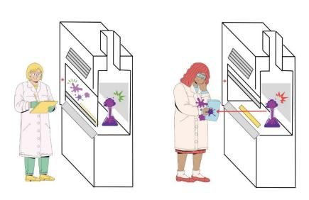
When using a fume hood, keep the sash at or below the line on the yellow certification sticker. Otherwise, close the sash completely to shield you and everyone in your lab from splashes and projectiles.
